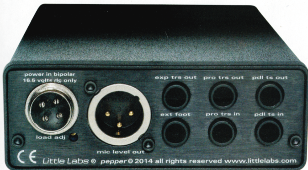
Fig. 2. Back-panel I/Os include XLR and balanced 1/4" outputs.
